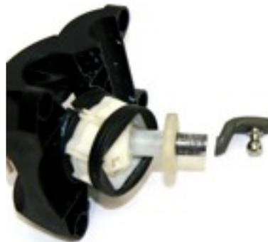
You should remove the cable coupler/adjuster from the original shifter in the car, it just pops off the ball. The shifter can be installed without readjusting the shifter mechanism this way but it can be beneficial to fine tune the adjustment afterwards. This is not as hard as it sounds, Really!
